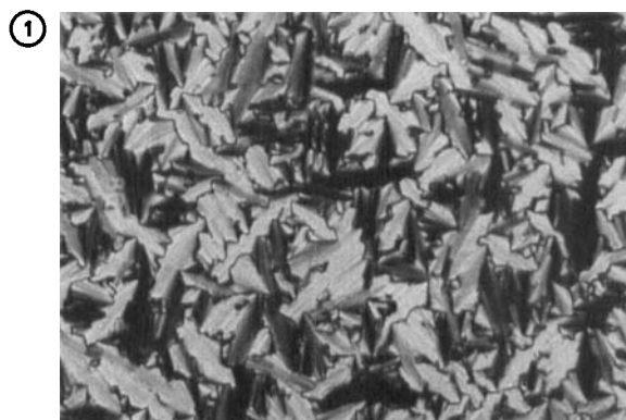
Typical fan-shaped smectic texture obtained with G24A90%, after a 24 hour annealing. Enlargement = 80.
